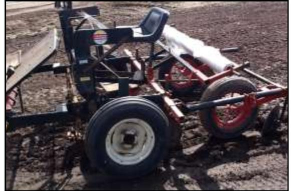
*This machine (above) puts a row tunnel wire in the ground and covers it with plastic. It takes about 20 minuets to put up a 230 foot row. Below, some of the tunnel rows after being covered by the "Tunnel Layer" machine.*
